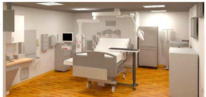
Increased size Trauma Room that includes medical equipment necessary for resuscitation, a negative pressure laminar flow system for infection control, and room enough to provide needed care for trauma situations.
